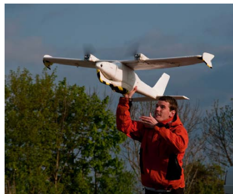
Figure 1. MAVinci Sirius I being launched by hand.
